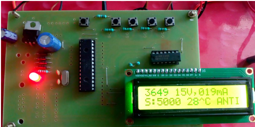
Figure 13 Indication of DC Motor Current
