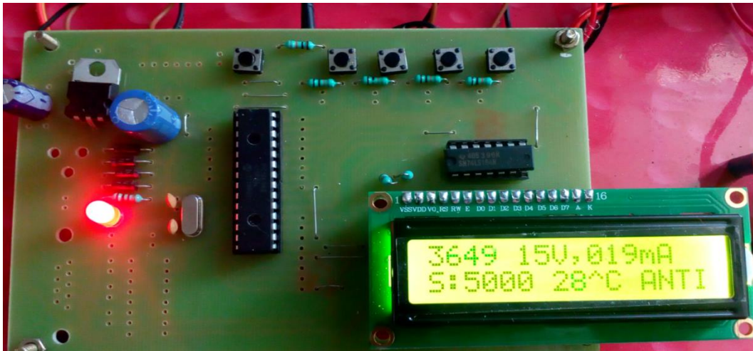
Figure 11 Indication of Motor Speed at 5000 rpm
